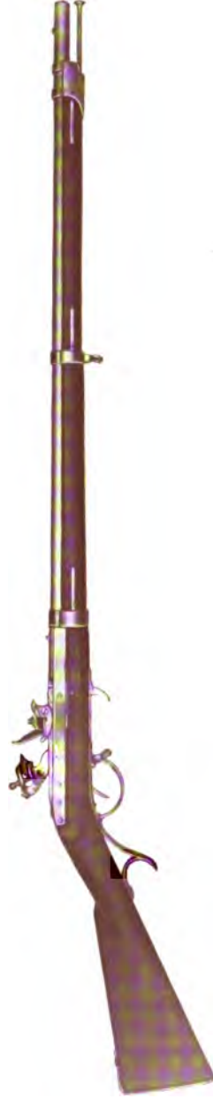
Hall Rifle. Length 52\frac{1}{2} inches. Length of barrel 32\frac{1}{2} inches. Depth of chamber in receiver 2\frac{1}{8} inches. Caliber, .54. Harper's Ferry model.
